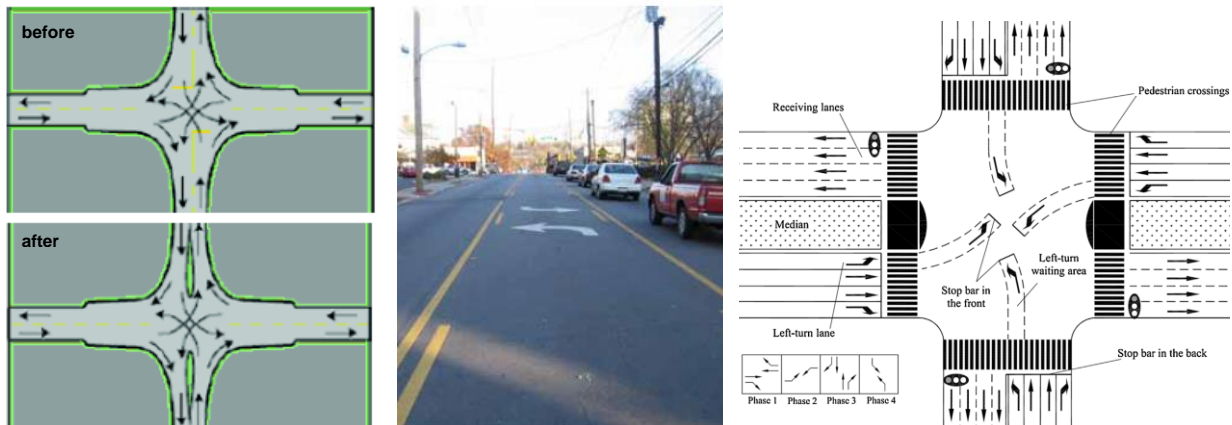
Figure 1. Junction channelisation before and after the installation of traffic islands on the main road – left (Yannis et al. 2011), center two-way left-turn lanes – middle (Persaud et al. 2007) and left-turn waiting areas – right (Jiang et al. 2016)
